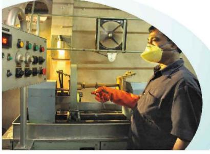
MPI test to detect cracks
