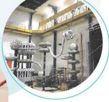
Dielectric test on 400kV Single Suspension fittings at Wuhan, China
